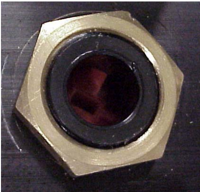
Pic. 15: Ventilation screw inside
