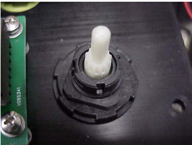
Pic. 14: UPPER part power circuit breaker
