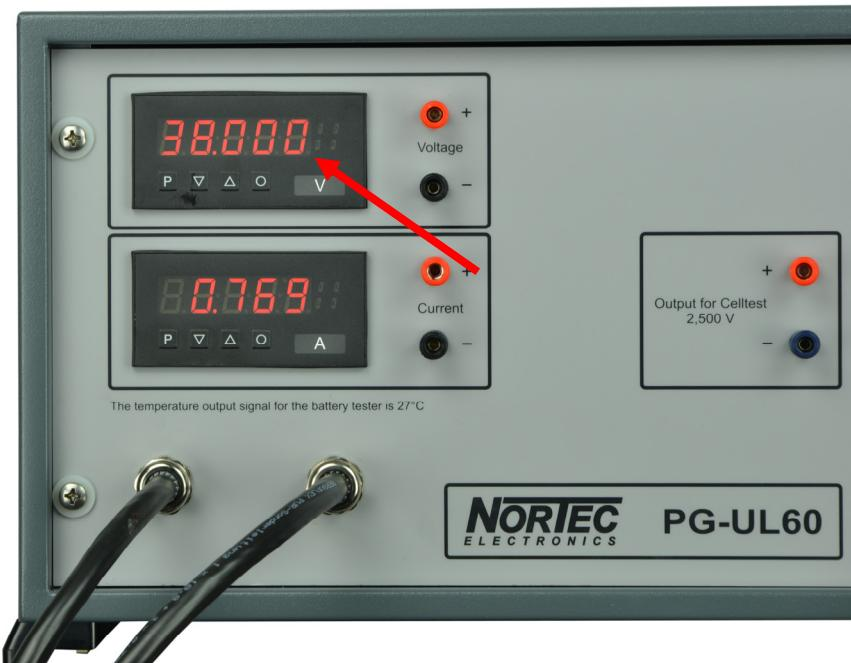
Fig. 3: Measurement calibration voltage 38 volts
