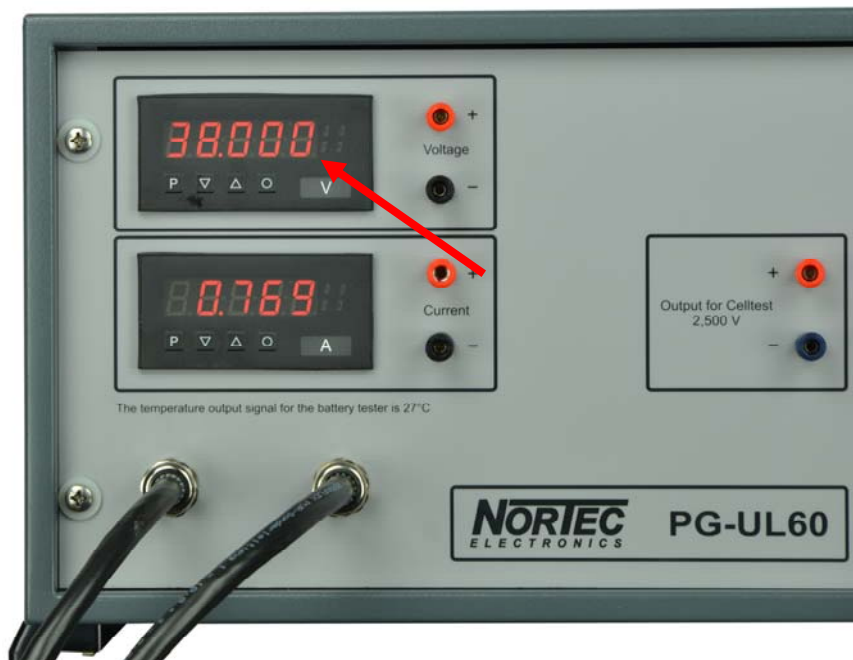
Fig. 3: Measurement calibration voltage 38 volts
