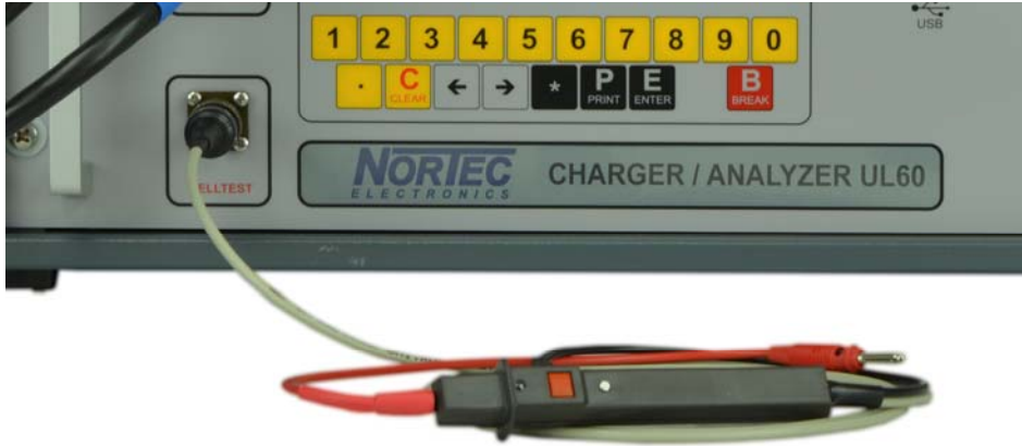
Fig. 7: Connected celltest 025D to the UL60
