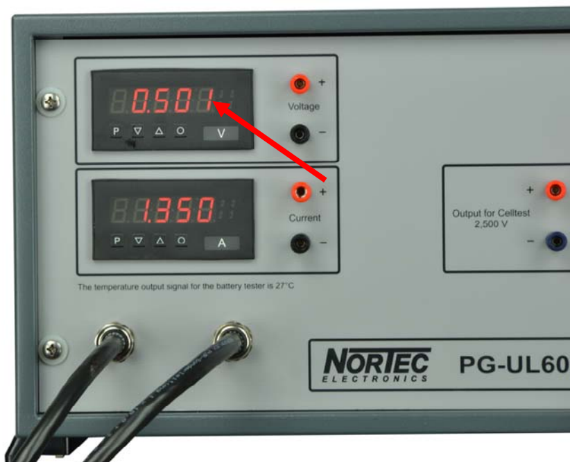
Fig. 2: Measurement calibration voltage 0.5 volts
